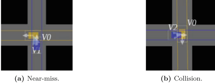
Fig. 4. Illustration of Safety-critical events. a) Near-miss: an occurrence where the safety distance between vehicles is compromised; b) Collision: an incident where the physical bodies of two or more vehicles come into contact.
