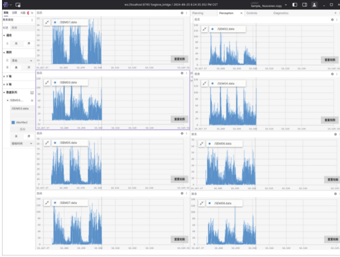
Fig. 3. 8-Channel Raw Surface EMG Signals Acquired by Myo.
