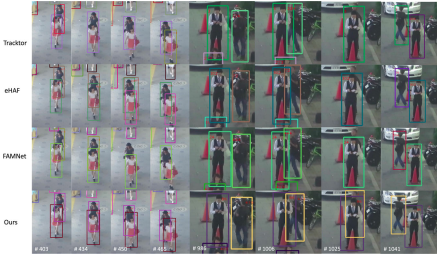
Fig. 6 An example of how our proposed approach (the last row) successfully handles a large overlapping case in MOT Challenge Video comparing with the state-of-the-art approaches Tracktor [1], eHAF [38], and FAMNet [9] (other rows). Best viewed in color
