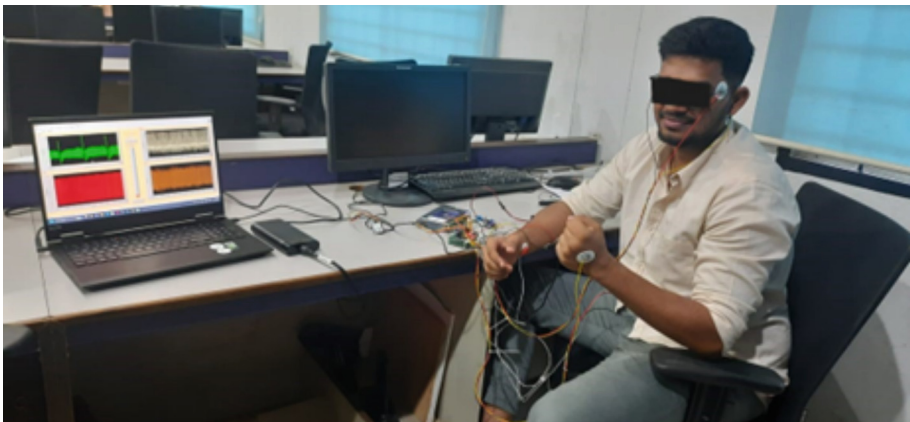
Fig. 5. Patient Biomedical Monitoring - Remote Care System LabVIEW hardware connection with patient
