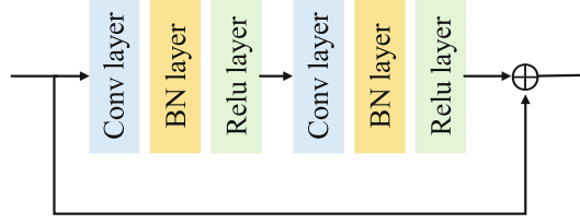
Fig. 3. The structure of Res-block
