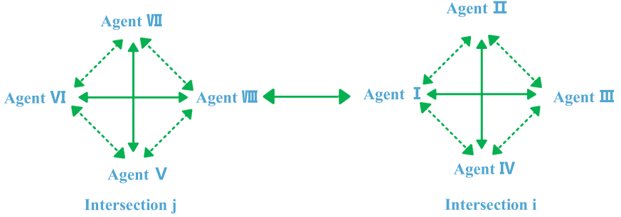
Fig. 3. Topology Structure of the Multi-Intersection System.
