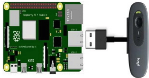
Fig. 5. Interfacing Camera with Raspberry Pi
