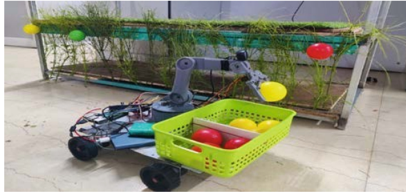
Fig. 10. Plucking and Segregation of yellow tomato.
