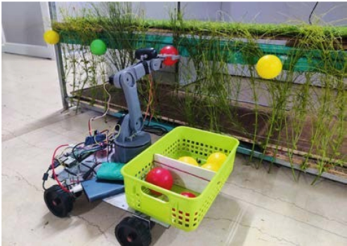
Fig. 8. Red colour tomato plucked by robot
