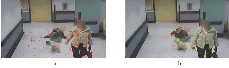
Fig. 2. Motion vectors in (a) MPEG-4 frame, and (b) H.264 frame. Borders of macroblock are white, while motion vectors in P and B frames are red and green, respectively. Macroblocks with no motion vectors are intra-coded.
